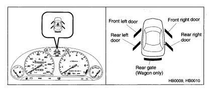
Your vehicle is equipped with door open warning lights. When a door is not fully closed, a light comes on indicating specifically which door it is. When all doors are properly closed, all of the door open warning lights go out. Always make sure these lights are out before starting to drive.
