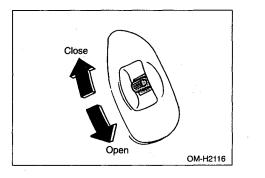
When the lock switch on the power window switch cluster, located on the driver's side door, is in the "LOCK" position, the passengers' windows cannot be operated with the passengers' switches.
