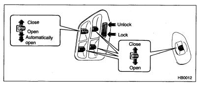
All door windows can be controlled by the power window switch cluster at the driver side door.
