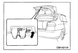
The inside trunk lid release can be cancelled to help prevent unauthorized entry into the trunk. To cancel the trunk lid release, set the lid release cancel lever (located on the inside of the trunk lid, mounted to the trunk lid latch) to the "CANCEL" position. When this lock is in the "CANCEL" position, the trunk can be opened only by the master key.
