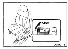
Pull the trunk lid release lever upward.
