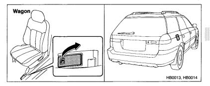
To open the fuel filler lid, pull the lid release lever up.
