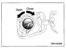
To take off the fuel filler cap, turn it counterclockwise slowly and remove the cap.
