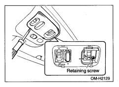
2. Remove the spot light lens by hand, then remove the switch body retaining screw and take off the sunroof switch.
