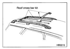
Luggage can be carried on the roof after securing the roof cross bar kit to the roof rail. When installing the roof cross bar kit on the roof rail, follow the manufacturer's instructions. The roof cross bar kit is designed to carry loads (luggage and roof rack) of not more than 100 lb. (45 kg).
