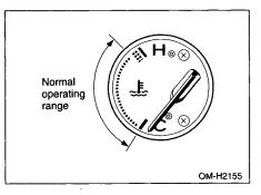
The temperature gauge shows engine coolant temperature when the ignition switch is in the "ON" position.
