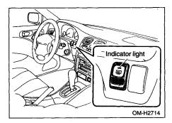
To turn on the defogger, push the switch. To turn it off, push the switch again.
