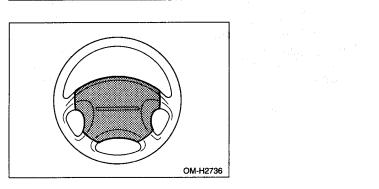
To sound the horn, push the horn pad.
