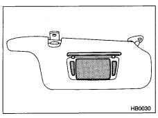
To use the vanity mirror, swing down the visor and open the cover. The lights beside the vanity mirror come on when the ignition switch is either in the "ACC" or "ON" position and the mirror cover is opened.
