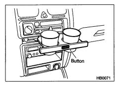
To use the cup holder, push the button and it will automatically pop out then pull it out completely.
