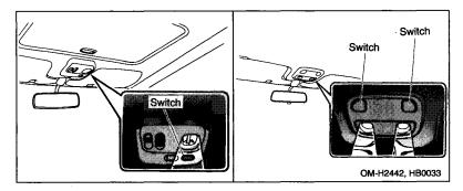
To turn on the spotlight, push the switch. To turn it off, push the switch again.
