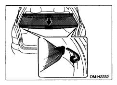
To extend the cover, pull the end of the cover out of the cover housing, then insert its hooks into the catches as shown. To rewind it, unhook it from the catches and it will rewind automatically.
