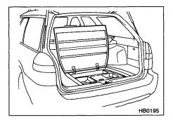
The storage tray is located under the floor of the luggage compartment and can be used to store small items. To open the lid, pull the handle up.
