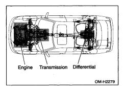
Inspect the following for oil leaks:
