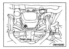
4. Drain out the engine oil by removing the drain plug while the engine is still warm. The used oil should be drained into an appropriate container and disposed of properly.
