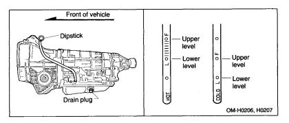
4. Pull out the dipstick and check the fluid level on the gauge. If it is below the lower level on the "HOT" side, add the recommended automatic transmission fluid up to the upper level.
