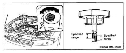
4. Remove the dipstick again and check the fluid level on it. If it is below the lower level of the "HOT" range, add the recommended steering fluid up to the specified range of the dipstick.
