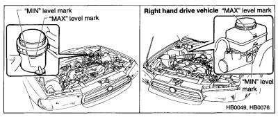
Check the fluid level on the outside of the reservoir. If the level is below "MIN", add the recommended brake fluid to "MAX".
