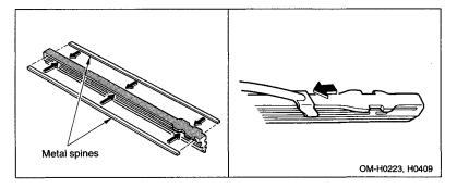
4. Be sure to position the end of the wiper blade between the stoppers on the rubber as shown. If the rubber is not retained properly, the wiper blade may scratch the windshield.
