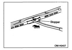
2. Pull out the blade rubber assembly while depressing the stoppers on the rubber.
