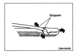
3. Install the new blade rubber assembly, aligning the claws of the blade with the grooves in the rubber.
