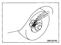
The front disc brakes and the right side rear disc brake have audible wear indicators on the brake pads. If the brake pads wear close to their service limit, the wear indicator makes a very audible scraping noise when the brake pedal is applied.
