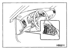
The fuses are designed to melt during an overload to prevent damage to the wiring harness and electrical equipment. The fuses are located in three fuse boxes.
