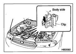
(1) Remove the four upper clips from radiator panel. To facilitate removal, press the portion shown in the illustration using screwdriver.
