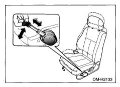
Pull the adjustment lever out and move it up or push it down to raise or lower the seat.
