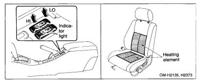
To turn on the seat heater, push the "LO" or "HI" position on the switch, as desired, depending on the temperature.
