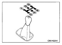
The shift pattern is shown on the shift lever knob. When shifting from 5th gear to reverse gear, first return the shift lever to the neutral position then
