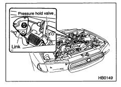
2. Find the Pressure Hold Valve. It is located inside the engine compartment under the brake fluid reservoir (big yellow cap).
