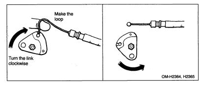
3. Turn the link clockwise to loosen the wire enough to form a loop.
