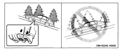
On an uphill grade, when the clutch pedal is depressed while the brake pedal is also depressed, braking power is maintained temporarily by the Hill Holder when the brake pedal is released. The driver is therefore able to start the vehicle the same way as on a level grade, just using the clutch and accelerator pedal.
