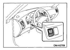
To turn off the TCS, push this switch while the engine is running. The indicator light on the switch will come on when the TCS is inactive. In this condition, the vehicle acts in the same way as a vehicle without TCS. Push this switch again to turn on the system.
