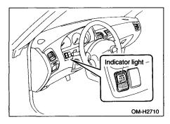
The TCS OFF indicator light comes on when the ignition switch is turned to the "ON" position and goes out within a few seconds after the engine starts. If the light does not come on when the ignition switch is turned "ON" and does not go out within a minute after the engine starts, it may indicate that TCS is not working properly. Contact your nearest SUBARU dealer immediately.
