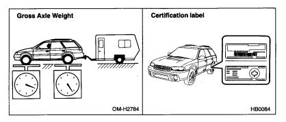
To check both GVWR and GAWR and to confirm that the total weight and weight distribution are within safe driving limits, you should have your vehicle and trailer weighed at a commercial weighing station. Be sure that all cargo is firmly secured to prevent a change in weight distribution while driving.
