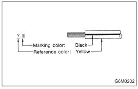
7) The wire color code, which consists of two letters (or three letters including Br or Lg), indicates the standard color (base color of the wire covering) by its first letter and the stripe marking by its second letter.
