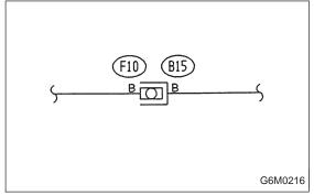
5) In wiring diagram, connectors which have no terminal number refer to one-pole types. Sketches of these connectors are omitted intentionally.
