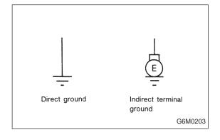
9) Each unit is directly grounded to the body or indirectly grounds through a harness ground terminal. Different symbols are used in the wiring diagram to identify the two grounding systems.
