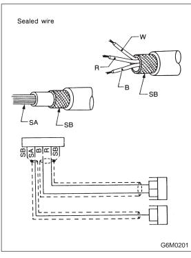
6) The following color codes are used to indicate the colors of the wires used.
