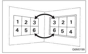
When one set of connectors is viewed from the front side, the pole numbers of one connector are symmetrical to those of the other. When these two connectors are connected as a unit, the poles which have the same number are joined.
