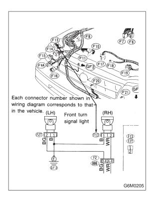
11) Each connector number shown in the wiring diagram corresponds to that in the wiring harness. The location of each connector in the actual vehicle is determined by reading the first character of the connector (for example, a "F" for F8, "i" for i16, etc.) and the type of wiring harness. The first character of each connector number refers to the area or system of the vehicle, as indicated in table below.
