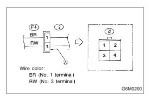
4) The sketch of each connector in the wiring diagram usually shows the "A" side of the connector. The relationship between the wire color, terminal number and connector is described in figure.
