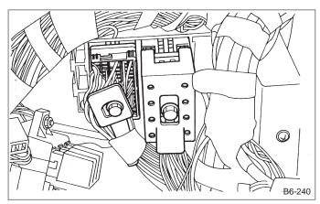
*Tightening torque:* 4.4 — 7.4 № m (45 — 75 kg-cm, 39 — 65 in-lb)
