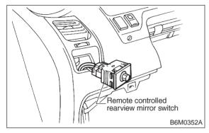
2) Remove rearview mirror switch while disconnecting connector.
