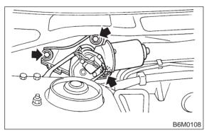
4) Remove wiper link from back side of wiper motor using a screwdriver inserted into service hole in front panel.
