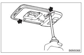
3) Remove room light body while disconnecting connector.
