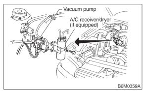
4) Remove vacuum pump while disconnecting vacuum hose.
