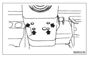
3) Remove screws which secure knee protector and remove knee protector.
