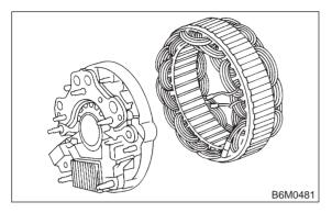
8) Remove bolts which secure IC regulator, diode and brush holder.
