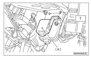
4) Remove cruise control module (A) while disconnecting connector.
