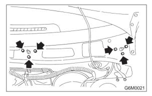
8) Remove wiper link from service hole in front panel.
