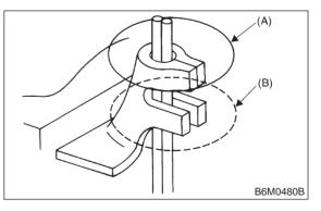
(3) Remove stator coil from diode plate.
