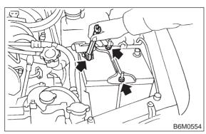
3) Remove washer tank mounting bolts.
