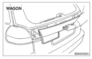
5) Attach adhesive cloth tape to body area around rear finisher.
