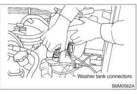
5) Move washer tank upward.
