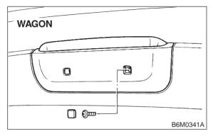
3) Remove high-mount stop light while disconnecting connector from body harness.
