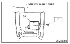
3) Remove security control module while disconnecting connector.
