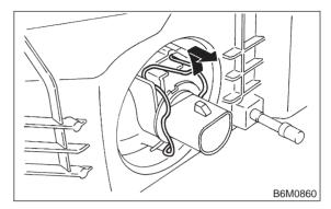
3) Replace the bulb with a new one and hook the spring.
