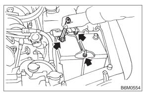
3) Remove washer tank mounting bolts.
