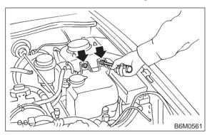
4) Disconnect washer tank connectors.
