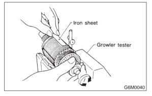
5) Armature ground test
