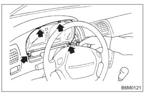
6) Disconnect connectors from back of combination meter.
