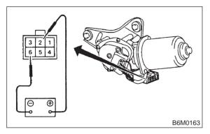
2) Check wiper motor operation at high speed: Connect battery to wiper motor. Check wiper motor for proper operation at high speed.
