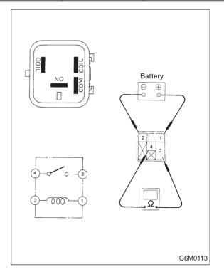
Check continuity between terminals (indicated in table) when terminal No. 1 is connected to battery and terminal No. 2 is grounded.
