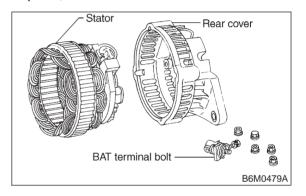
7) Separate diode plate from stator coil.(1) Cut the connecting position (A) of stator coil to diode.
