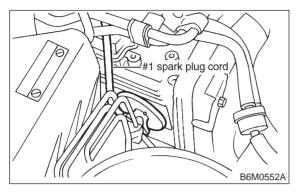
3) Remove spark plug with the spark plug socket.
