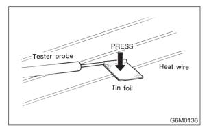
4) When tester indicates 12 volts when its probe reaches point "A", a broken circuit occurs between point "A" and the negative terminal. Slowly move tester probe toward the negative terminal while contacting it on heat wire to locate point where tester indication changes abruptly (0 volts). This is the point where a broken circuit occurs.
