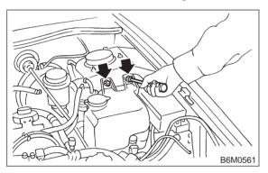
4) Disconnect washer tank connectors.
