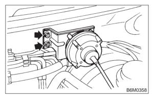
4) Remove actuator while disconnecting vacuum hose.
