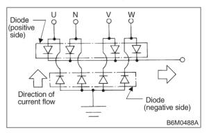
1) Diodes on "+" side Continuity of proper diodes on "+" side
