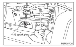
7) For subsequent procedures, refer to the procedure for #1 spark plug. <Ref. to 6-1 [W3C1].>
