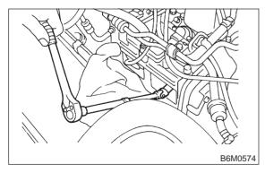
8) The subsequent procedures are in reverse order of #1 spark plug removal. <Ref. to 6-1 [W3C1].>
