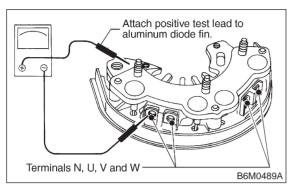
2) Diodes on "–" side Continuity of proper diodes on "–" side
