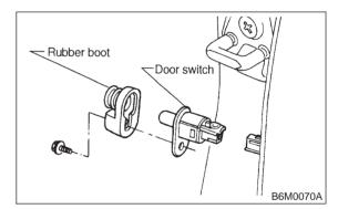
3) Remove door switch while disconnecting connector.
