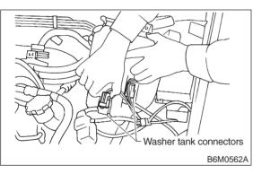
5) Move washer tank upward.
