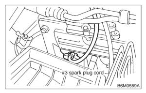
7) Remove spark plug with the spark plug socket.
