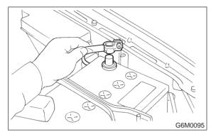
2) Disconnect mass air flow sensor connector.
