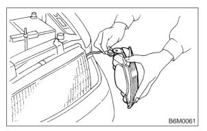
4) Remove bolts which secure headlight and remove headlight.
