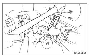
5) When installing, tighten the connecting bolt until its head twists off.
