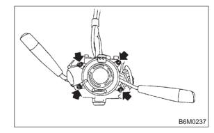
2) Remove screws which secure lighting switch, wiper and washer switch. Remove both switches.3) Assembly is in the reverse order of disassembly.
