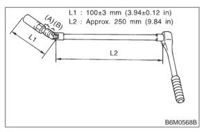
9) Set (D) extension and (E) ratchet in turn onto the connected tools in plug hole, and remove spark plug using them.
