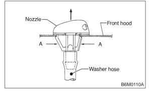
3) Remove nozzle from engine hood.
