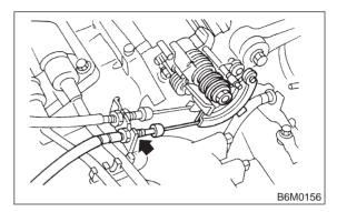
3) Remove nuts which secure actuator.
