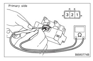
[Secondary side] Between (A) and (B) 12.8 kΩ±15% Between (C) and (D) 12.8 kΩ±15%
