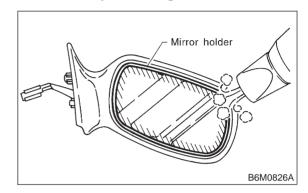
3) Remove mirror plate while lifting the mirror holder using a flat bladed screwdriver.
