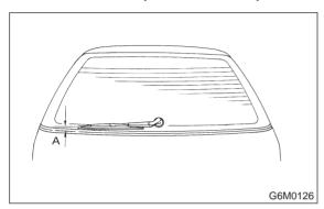
2) Adjust washer ejecting point on rear gate window as shown in figure when the vehicle stops.
