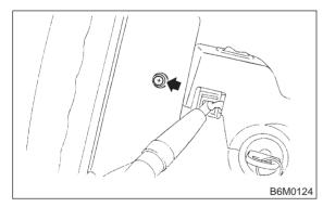
2) Remove horn switch (steering pad) from steering wheel while disconnecting connector.
