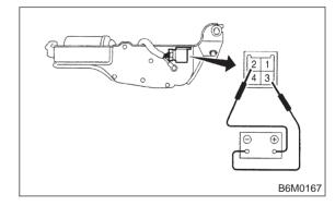
2) Check wiper motor for proper stoppage: After operating wiper motor, disconnect battery from wiper motor.
