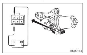
3) Check wiper motor for proper stoppage:
