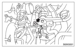
5) Disconnect connector and terminal from starter.
