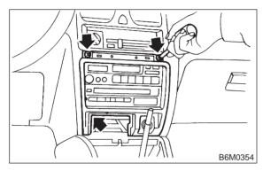
4) Remove fitting screws, and slightly pull radio out of instrument panel.
