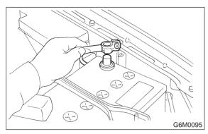
2) Disconnect mass air flow sensor connector.
