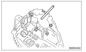
• When installing rear cover, heat portion (A) to 50°C (122°F) with heater drier.
