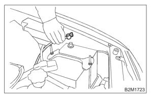
2) Disconnect connector and terminal from generator.
