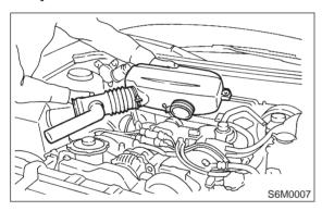
3) Remove air intake chamber stay. (AT vehicles only)
