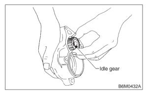
13) Remove retainer and roller from housing.
