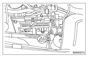
3) When spark plug is screwed in two or three turns, temporarily disconnect the tools connected in the first step.
