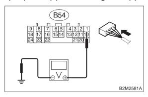
CHECK : Is the voltage less than 1 V in "1" range?
