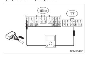
: Is the resistance less than 1  $\Omega$ ? (CHECK)
