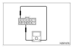
CHECK : Is the resistance less than 1  $\Omega$  in "D" range?
