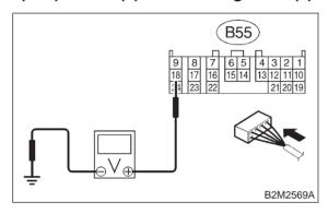
CHECK : Is the voltage less than 1 V in "3" range?
