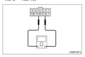
CHECK : Is the resistance less than 1  $\Omega$  in "P" range?
