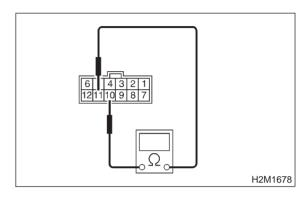
: Is the resistance less than 1  $\Omega$  in "2" CHECK range?
