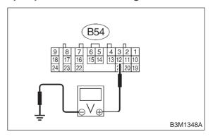
CHECK : Is the voltage less than 1 V in FWD switch while installing?
