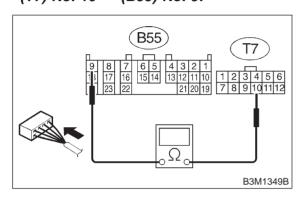
(CHECK): Is the resistance less than 1  $\Omega$ ?
