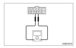
CHECK : Is the resistance less than 1  $\Omega$  in "R" range?
