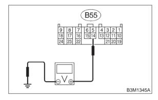
: Is the voltage less than 1 V in FWD CHECK switch while installing?
