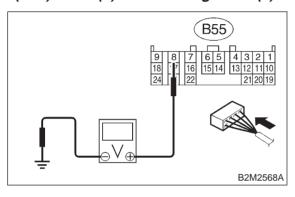
CHECK : Is the voltage less than 1 V in "D" range?
