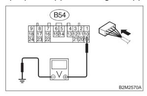
CHECK : Is the voltage less than 1 V in "2" range?
