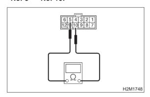
CHECK : Is the resistance less than 1  $\Omega$  in "N"
