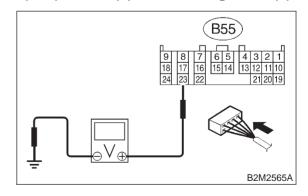
CHECK : Is the voltage less than 1 V in "P" range?
