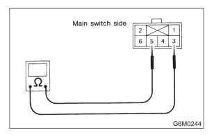
CHECK : Is resistance less than 10  $\Omega$ ? (When
