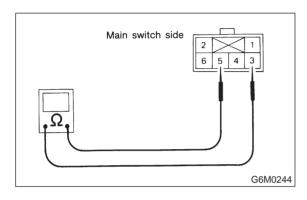
CHECK : Is resistance more than 1 M $\Omega$ ? (When switch is OFF.)
