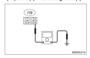
(CHECK): Is resistance less than 10  $\Omega$ ?
