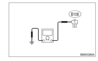
(CHECK) : Is the resistance less than 10  $\Omega$ ?
