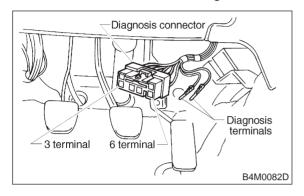
2) Repeat 3 times within approx. 12 seconds; connecting and disconnecting terminal 6 and diagnosis terminal for at least 0.2 seconds each time.
