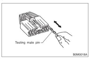
5) Shake lightly the connector and the harness, and check for sudden changes in voltage or resistance.
