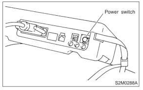
3) Disconnect test mode connector at the lower portion of instrument panel (on the driver's side), to the side of the center console box.
