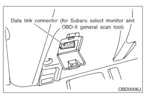
3) Turn ignition switch to ON and Subaru Select Monitor or OBD-II general scan tool switch to ON.4) Start engine.
