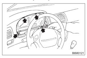
3) Disconnect connector from combination meter.
