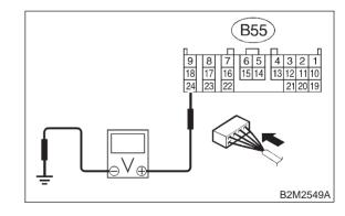
CHECK : Is the voltage less than 1 V when releasing the brake pedal?
