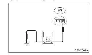
: Is the resistance less than 5  $\Omega$ ? CHECK
