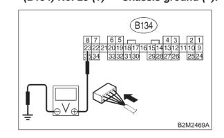
CHECK : Does the voltage change less than 1.0 V by shaking harness and connector of ECM while monitoring the value with voltage meter?
