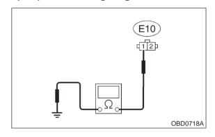
: Is the resistance less than 10  $\Omega$ ? CHECK
