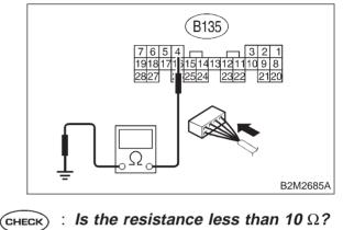
**YES** : Repair ground short circuit in harness between ECM and TCM connector.
