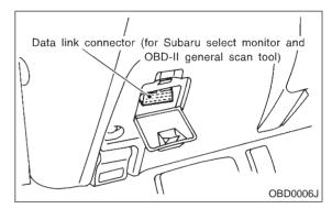
3) Turn ignition switch to ON and Subaru Select Monitor or the OBD-II general scan tool switch to ON.
