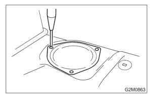
Disconnect connector from fuel sub meter unit.
