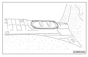
3) Disconnect connector from fuel pump.
