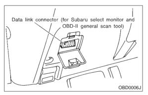
3) Turn ignition switch to ON and Subaru Select Monitor or OBD-II general scan tool switch to ON.4) Start engine.
