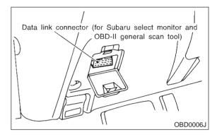
4) Turn ignition switch to ON and Subaru Select Monitor or OBD-II general scan tool switch to ON.
