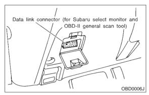
5) Turn ignition switch to ON and Subaru Select Monitor or the OBD-II general scan tool switch to ON.
