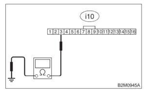
(CHECK) : Is the resistance less than 200  $\Omega$ ?
