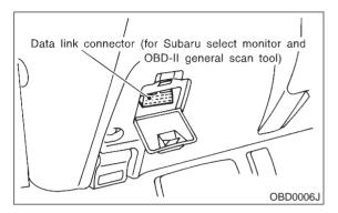
3) Turn ignition switch to ON and Subaru Select Monitor switch to ON.
