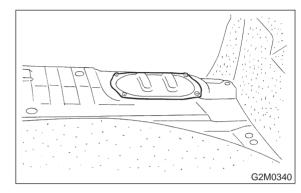
Disconnect connector from fuel pump.
