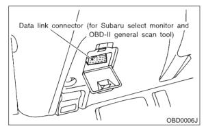
3) Start the engine, and turn Subaru Select Monitor or OBD-II general scan tool switch to ON.
