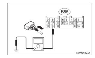
$\overline{\text{CHECK}}$  : Is the resistance more than 1 M $\Omega$ ?
