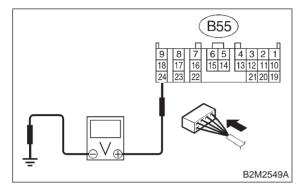
CHECK : Is the voltage more than 10 V when depressing the brake pedal?
