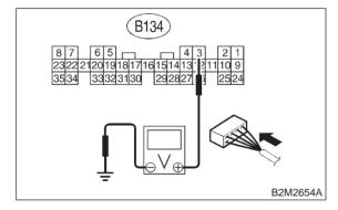
CHECK : Does voltage change between 0 and 10 volts?
