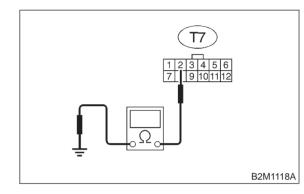
: Is the resistance less than 5  $\Omega$ ? CHECK
