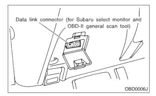
3) Turn ignition switch to ON and Subaru Select Monitor or the OBD-II general scan tool switch to ON.
