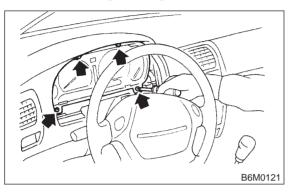
Disconnect connector from combination meter.
