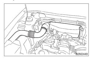
3) Remove engine harness connector bracket from cylinder block.
