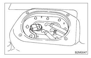
3) Disconnect fuel delivery hose from fuel filter, and connect fuel pressure gauge.
