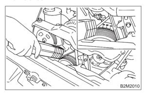
If the timing is not correct, check the ignition control system. <Ref. to 2-7 [T6A0].>
