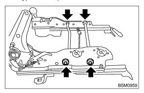
29) Remove 2 bolts, and then remove slide rail. (Non-tilt type vehicle)
