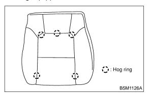
11) Remove wire rings, and then remove seat heater. (Seat heater equipped vehicle)
