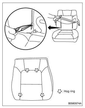
Side airbag equipped vehicle:
