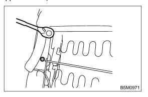
16) Remove the 4 bolts of seat hinge assembly, and then remove seat cushion.
