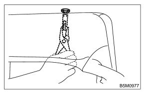
10) Remove wire ring on front face of seat.
