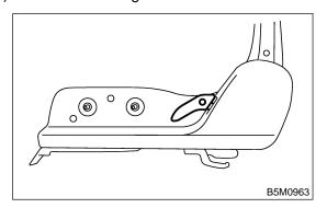
25) Remove hinge cover cap and screws.
