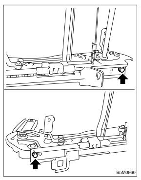
28) Remove 4 screws, and then remove hinge. (Non-tilt type vehicle)
