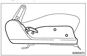
17) Remove the 4 bolts of seat hinge assembly, and then remove seat cushion. Tilt type vehicle:
