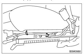
7) Turn cover and cushion, and remove the two bolts from hinge.
