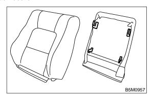
4) Remove hook on back side of seat, and remove hog rings using a plier.
