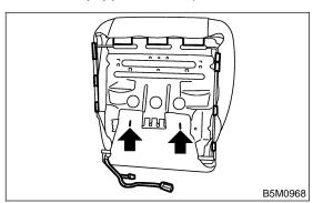
20) Remove hog rings. Tilt type vehicle:
