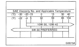
The proper viscosity helps vehicle get good cold and hot starting by reducing viscous friction and thus increasing cranking speed.
