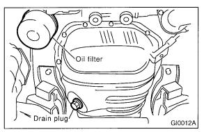
2) Get a new oil filter and apply a thin coat of engine oil to the seal rubber.
