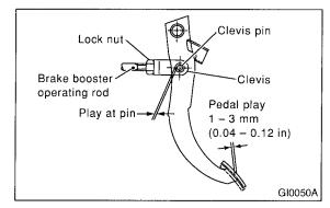
2) If the free play is out of specifications above, adjust the brake pedal as follows:
