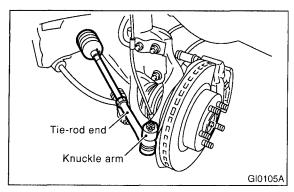
2) Check connections of knuckle ball joints for play, inspect for damage on dust seals, and check free play of ball studs. If castle nut is loose, retighten it to the specified torque, then tighten further up to 60° until cotter pin hole is aligned.
