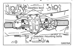
2) Check boot for damage, cracks or deterioration.
