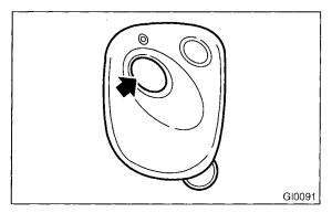
• Press the "UNLOCK/DISARM" button on the transmitter momentarily once and check if the driver's door is unlocked, the horn chirps twice and the dome light illuminates.
