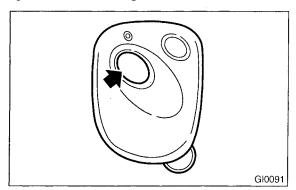
• Press the "UNLOCK/DISARM" button on the transmitter momentarily once and check if the driver's door is unlocked, the horn chirps twice, the parking lights flash twice, the dome light illuminates and the security indicator light goes off to ensure that the system has been brought into the disarming state.
