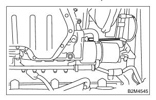
6) Remove oil pressure switch.
