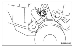
3) Connect terminal of oil pressure switch.
