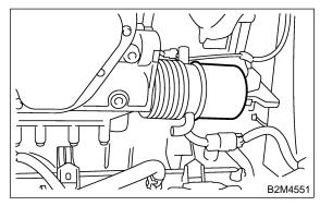
8) Remove connector and remove oil cooler.
