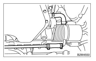
4) Install water pipe to engine.
