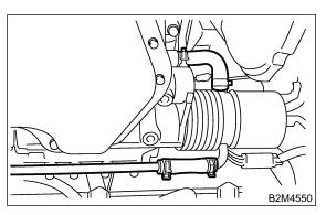
7) Remove oil filter using ST. <Ref. to LU(H6)-18, REMOVAL, Engine Oil Filter.>
