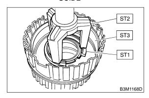
6) Install the dish plate, driven plates, drive plates, and retaining plate, and secure with the snap ring.
