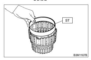
5) Set the cover on the piston with a press using ST1 and ST2, and attach the snap ring.
