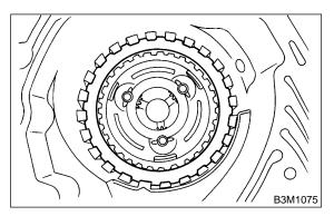
17) Take out the thrust needle bearing, planetary gear assembly and the low clutch assembly.
