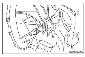
14) Install the torque converter clutch assembly. <Ref. to AT-35, INSTALLATION, Torque Converter Clutch Assembly.>
