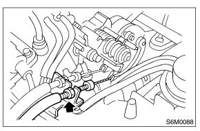
4) Remove actuator attaching bolts.
