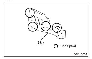
3) Remove main switch by pushing it outward.
